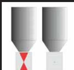
Femtosecond lasers excite the fluochrome only at the focus.
