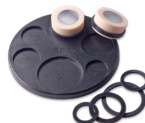
Levelling tool for adjusting retention rings on individual specimens for Lavamin.
