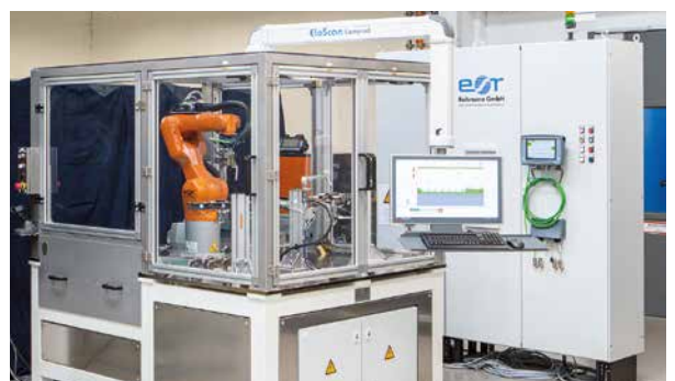
Robot controlled inspection system with ELOTEST PL650, ELO\SCAN and image processing module ELO\IMAGE.
