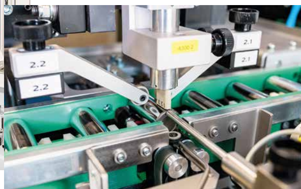
Automated inspection for cracks and grinding burns on rolling elements with the ELOTEST PL650 and probes (Type KD-129 and KDA-129).
