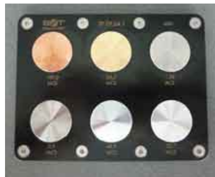
Reference standard TP79.04.1 Conductivity standard
