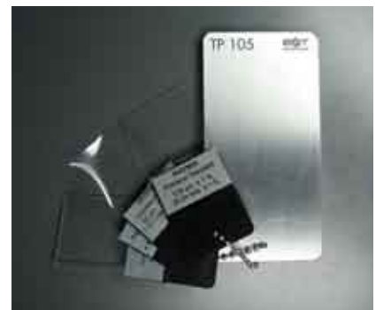
Reference standard TP 105 aluminium Coating thickness standard
