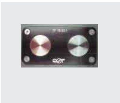
Reference standard TP 79.02.1 Conductivity standard
