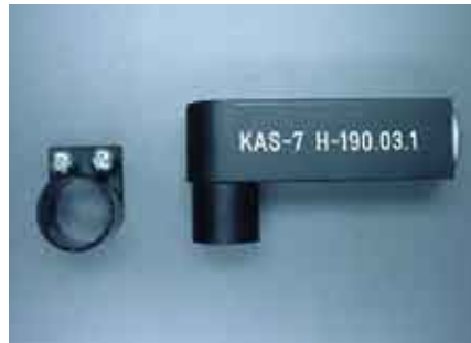
Probe with prism guiding KAS-7 H-190.03.1 Angled standard probe for conductivity measurement at 60 kHz
