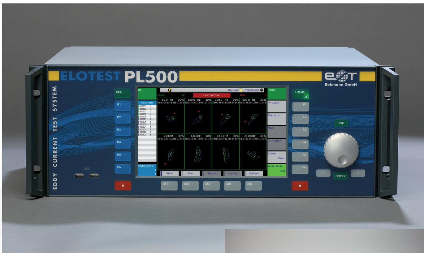
**Multi-frequency sorting inspection using the PL500Q has proven itself in practice. It combines simple operation by means of an automatic learning process with the security that nothing will be overlooked. A "fingerprint" of the learned good parts is generated using up to eight test frequencies. All other parts are compared to this, ensuring that deviations are found in terms of material, heat treatment or other test object properties that can be detected by electromagnetic means.**
