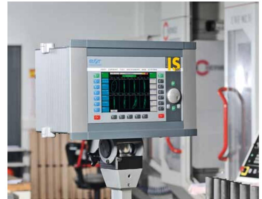
**The main feature of the new family of instruments is the fully digital signal processing chain with an extremely wide bandwidth starting from 10 kHz and with an ultra-fast multiplexing rate of a 32 kHz (probe to probe). The full dynamics of 96 dB across a frequency range of 10 Hz to 12 MHz speaks for itself.**
