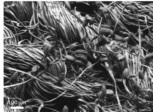
BSD image of pollen caught on fabric at a pressure of 58 Pa in water vapor at 20 kV.
